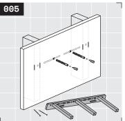
Predrill each drywall anchor location with a ¼" drill bit to avoid breaking drywall anchors. Install a drywall anchor in each of these pre-drilled locations. If you are using your own anchors, we recommend Toggler brand for best results. Stud locations should not be pre-drilled. Drywall anchors should be installed flush with the drywall surface with the drywall surface.
