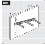
Let's dive in, homies! Orient your bracket on the wall so the channels across the top of your bracket face up. Use a drill to install a fastener in either far left or right
