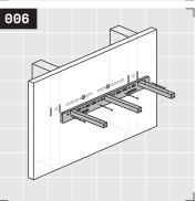
Confirm the position of the bracket and install a fastener into every location crossing a stud or blocking. For every location that a drywall anchor was installed, ensure a fully threaded #8 fastener is used.
