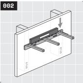
Level your bracket, set another fastener in the opposite end hole with your drill. If you have installed blocking behind the full length of your bracket, skip to **Step** 6. If you have not installed blocking, proceed to step 3. For more information on blocking, see **Rad Tip** ① on page 7.
