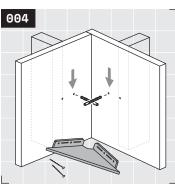
Use a stud finder to locate any available studs behind the drywall. For all remaining fastener locations, use a 1/4" drill bit to predrill each drywall anchor location.
