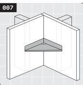
Snap the magnetic cover plate into place. Make a final inspection of your shelf. Check for shelf sag, confirm shelf is correctly secured to wall. See **Rad Tip** @ on page 7.
