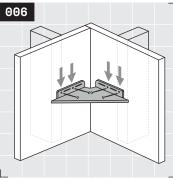
Replace the shelf and install a fastener into every drywall anchor and stud location.
