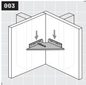
Double check the shelf position on your wall and adjust if necessary. Mark all fastener holes with a pencil. Once every fastener location has been marked, uninstall both fasteners and remove your shelf from the wall. Take a swig of your favorite soda or non-alcoholic brew.
