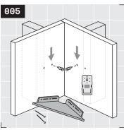
Install a drywall anchor in each of these pre-drilled locations. If you are using your own anchors, we recommend Toggler brand for best results. Stud locations should not be pre-drilled. Drywall anchors should be installed flush with the drywall surface.
