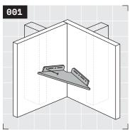
Yo! Here we go! Position your shiny new shelf in the corner of your wall with the fastener holes along the top edge. Use a drill to fasten either the far left or right hole to the wall in the desired location. For masonry installs, see Rad Tip ③ on page 7.
