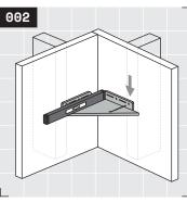
Level your shelf, then set another fastener in the opposite side with your drill. If you have installed blocking behind the full length of your shelf, skip to step 6. If you have not installed blocking, proceed to step 3. For more information on blocking, see Rad Tip ① on page 7.
