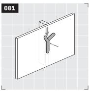
Yo, let's go! Position your Why Not hook on your wall in the desired location. Use a drill to install one of the included 1½" fasteners into the top fastener hole location.
