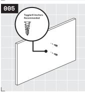
Install a wall anchor into both fastener locations. If you are using your own anchors, we recommend Toggler brand for best results.
