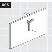
If your hook is on studs or blocking, install second 1½" fastener in lower marked location and proceed to step 7. For more information on studs and blocking, see Rad Tip ① on page 7.
