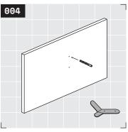
Remove your hook from the wall. Using a 1/4" drill bit, predrill both fastener locations.
