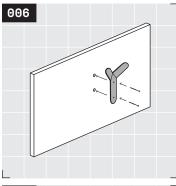
Replace your hook and make final install of the top and bottom matching 1½" fasteners.
