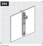
Replace your hanger and make final install of all matching truss head fasteners.
