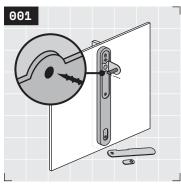
Yo, let's get started! Remove steel cover plates, and set aside. Your Wallride Vertical Bike Hanger features a bracket that can have the hook on either the right or left, so if you would like to switch the side that the hook is on, see Rad Tip ① on page 7.
