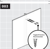
Remove your hanger from the wall. Using a 1/4" drill bit, predrill all fastener locations not on studs or blocking.
