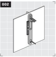
Use a level to vertically level your hanger. Mark remaining fastener hole locations with a pencil or fastener tip.
