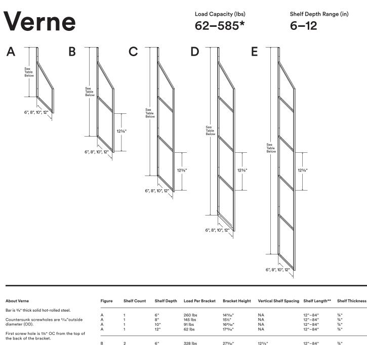
Each additional back bar screw hole is 21/2" OC above each shelf support bar.
