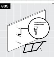
Remove the brackets from your wall. Predrill all marked fastener locations with a ½" drill bit, and install drywall anchors in each fastener hole location crossing drywall that isn't backed by studs or blocking. If you are installing on masonry, you must use a wall anchor rated for masonry use. If you are using your own anchors, we recommend Toggler brand. Take a swig of your brew.
