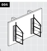
Install wall fasteners in the top fastener hole locations. Vertically level each bracket. Punch a hole in all remaining fastener locations with fastener tip. If your brackets are not on studs or blocking, skip to step 6. If your brackets are on studs or blocking, proceed to step 5.
