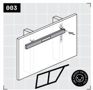
Place a level on first fastener hole. Find the intersection of the level and vertical line. If you do not have a long enough level, see **Rad Tip** ③ on page 7. Use a wall fastener to punch a hole into wall behind low-tack tape. Remove the tape.
