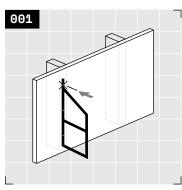
Yo, here we go! Position the first Verne bracket on your wall, ideally on a stud or blocking. See Rad Tip ① on page 7 if you don't know what blocking is. Mark the top-most fastener hole with the fastener tip. Remove bracket from wall, then grab a can of your favorite non-alcoholic brew and crack it open.
