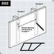
Measure the desired bracket spacing from fastener hole and righteously apply low-tack tape to general mounting area of second bracket. Measure again and draw a short vertical line on the tape. See Rad Tip ② on page 7.
