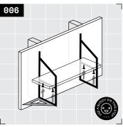
Position the brackets, install all 2" wall fasteners. Confirm the brackets are secure to wall. (Brackets may wiggle left to right at this point. Chillax, installing the shelves will resolve this!) Lay the top shelf on your bracket and position as desired. See Rad Tip @ on page 7. Position the brackets perpendicular to your wall by using a square. Hold the shelf in place and install all 1" shelf set screws, then repeat for remaining shelves. Take another swig of that sweet, sweet nectar.
