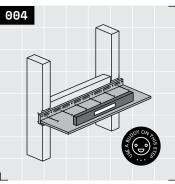
Reposition your shelf. Use a drill to fasten either far left or right hole, then level the shelf. Fasten second fastener in the opposite end fastener hole, then fasten all remaining fastener holes. Use shims to level as needed. Use a buddy to help on this step!
