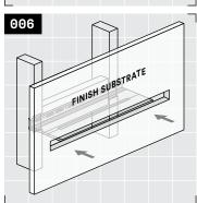
Carefully reinstall your finish substrates to align with the top and bottom of your shelf and secure to studs.
