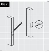
Mark a ¼" easement above and below the existing pencil line. Using a chisel or multitool, notch out each stud ¼" deep. Notches must be square and level.
