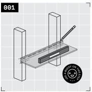
Here we go, homies! Remove any drywall to reveal the wall's studs in the install area. Position your shelf as desired and level. Mark all intersecting studs along the top and bottom edges of your shelf. It helps to have a buddy hold the shelf during this step! For masonry installs, see Rad Tip ③ on page 7.
