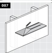
When finished, carefully use a blade or box cutter to remove the protective tape and masking paper, revealing your super crisp shelf!
