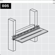
Make final inspection of your shelf, checking for shelf sag. Confirm the shelf is correctly and soundly secured to studs and blocking.
