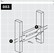
Install wood blocking between each stud in order to provide complete support for your shelf. See **Rad Tip** ①. Face of blocking should be flush with stud notches. For more information on making sure your shelf is flush and square, see **Rad Tip** ②. Secure blocking with fasteners from the side of the stud (A), or predrill with a ¾" drillbit and install pocket fasteners if the sides are not accessible (B).
