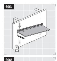
Yo! Here we go! Position your shelf on the wall with the pre-drilled holes along the top edge. Use a drill to fasten either the far left or right hole to the wall in the desired location. Using the slots will allow you to make minor adjustments to the position of your shelf. For masonry installs, see **Rad Tip** ③ on page 7.
