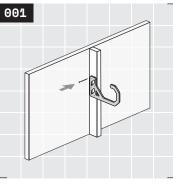
Yo! Here we go! Your Studly Hook is designed to be installed directly onto wall studs. See Rad Tip ① on page 7 for more information. Position your hook on a stud or post, then install a wall fastener into an upper fastener hole location.
