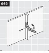
Straighten your hook using a level. Mark a lower fastener hole location with a fastener tip or a pencil. Install a second wall fastener into this location, then recheck for level.
