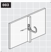
Install the remaining fasteners into remaining fastener holes. Your first Studly hook is installed! Crack open and take a swig of your favorite non-alcholic brew.
