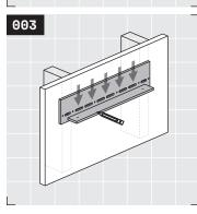
Double check the bracket position on your wall and adjust if necessary. Mark all fastener holes and slots with a pencil. Once every fastener location has been marked, uninstall both fasteners and remove your bracket from the wall. Take a swig of your favorite soda or non-alcoholic brew.
