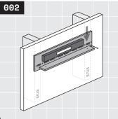
Level your bracket, then set another fastener in the next stud or opposite side with your drill. If you have installed blocking behind the full length of your bracket, skip to step 6. If you have not installed blocking, proceed to step 3. For more information on blocking, see Rad Tip ① on page 7.
