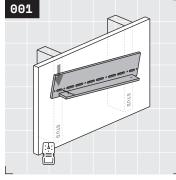
Yo! Here we go! Position your bracket on the wall with the pre-drilled holes and blade along the bottom edge. Use a drill to fasten either the far left or right hole to the wall in the desired location. Using the slots will allow you to make minor adjustments to the position of your bracket. For masonry installs, see Rad Tip ® on page 7.
