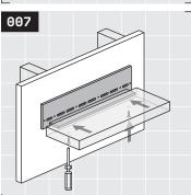
Slide wood shelf onto bracket. Install set screws with phillips screwdriver. Do not use power drill for set screw installation.
