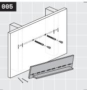
Predrill each drywall anchor location with a ¼" drill bit to avoid breaking drywall anchors. Install a drywall anchor in each of these pre-drilled locations. If you are using your own anchors, we recommend Toggler brand for best results. Stud locations should not be pre-drilled. Drywall anchors should be installed flush with the drywall surface.
