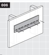
Replace the bracket and install a Truss head fastener into every location crossing a stud or blocking. For every location that a drywall anchor was installed, ensure a fully threaded #8 pan head fastener is used. For more information on fasteners, see **Rad Tip** @ on page 7.
