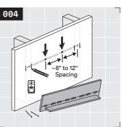
Use a stud finder to mark the location of every stud the bracket crosses. Then for areas between studs, mark a drywall anchor install location roughly every four to six inches along the length of the bracket.
