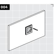
Confirm that your hook is on the wall in the desired location. Mark upper fastener hole with pencil or fastener tip. Predrill marked location with ¼" drill bit, making a pilot hole for a wall anchor.
