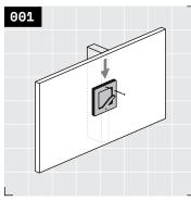
Yo, let's go! Position your Shingle hook on your wall in the desired location. Align the top fastener hole with wall area backed by a stud or blocking. See **Rad Tip** ① on page 7 for more information on blocking. Use a drill to install one of the included 1½" fasteners into this location. If there is no stud or blocking, skip to step 4.
