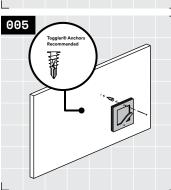
Install a wall anchor into the fastener hole, then install your hook and first 11/2" fastener. Fasten less than full tightness.
