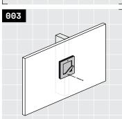
Install second 11/2" fastener in lower marked location. If your hook is on studs or blocking, proceed to step 4.
