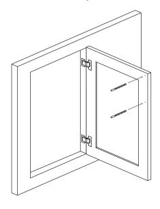
Reposition your cabinet pull, and install cabinet screws with a phillips head screw driver.
