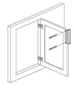
Drill a small pilot hole in the center of your mark with a #44 (.086") or smaller drill. To avoid accidental drill through, keep the pilot hole shallow.
