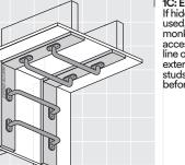
1C: External studs or blocking If hidden structural elements cannot be
