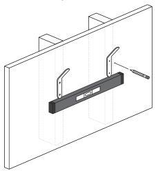
Install upper screw into marked location. Check for level, and install remaining screw into lower screw hole. Repeat for additional hooks. Skip to step 9.
