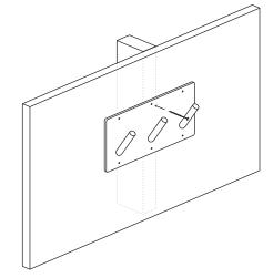
Postion the hook in desired location. Use a drill to install a wall fastener screw into an upper screw hole.
