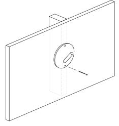
Level the hook by vertically aligning the upper and lower screw holes, use bullet level if needed. Mark lower hole with pencil or screw tip.
