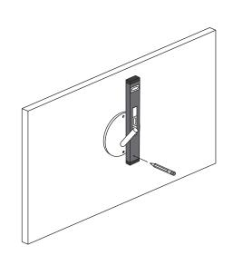
Uninstall wall hook. Drill a pilot hole 6 in both screw locations with a 1/8" drill bit. Install wall anchors in each hole.
