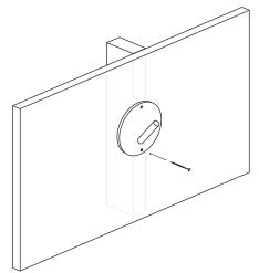
Position the hook in desired location. Use a drill to install a wall fastener screw into the upper screw hole.
