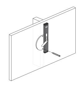
Install lower fastener screw into marked location. Skip to set 9.
