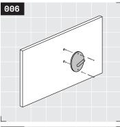
Replace your hook and make final install of the top and bottom matching 11/2" fasteners.
