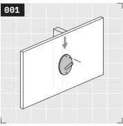
Yo, let's go! Position your Peggy Wall hook on your wall in the desired location. Use a drill to install one of the included 1½" fasteners into the top fastener hole location.
