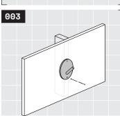
If your hook is on studs or blocking, install second 1½" fastener in lower marked location and proceed to step 7. For more information on studs and blocking, see Rad Tip ① on page 7.
