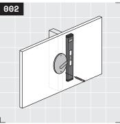
Use a level to vertically level your hook. Mark the lower fastener hole location with a pencil or fastener tip.
