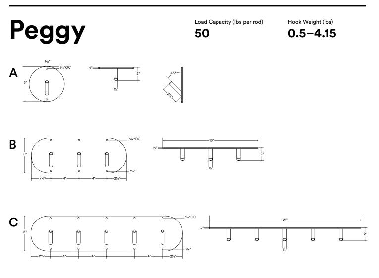
Backplate made from  $\mathcal{V}_4$ " thick hot-rolled steel.
