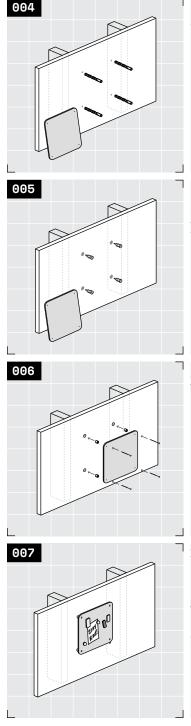
Drill a pilot hole for each fastener location using a  $\frac{1}{2}$ " drill bit. Pilot holes and wall anchors are not needed for locations backed by studs or blocking.
