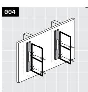
Install wall fasteners in the top fastener hole locations. Vertically level each bracket. Punch a hole in all remaining fastener locations with fastener tip. If your brackets are not on study or blocking, skip to step 6. If your brackets are on studs or blocking, proceed to step 5.
