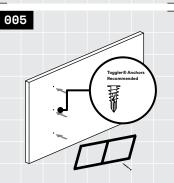
Remove the brackets from your wall. Predrill all marked fastener locations with a ¼" drill bit, and install drywall anchors in each fastener hole location crossing drywall that isn't backed by studs or blocking. If you are installing on masonry, you must use a wall anchor rated for masonry use. If you are using your own anchors, we recommend Toggler brand. Take a swig of your brew.
