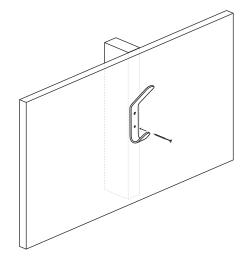
Position your next hook over a wall area backed by a stud or blocking. Use a level to align your hooks. See Rad Tip #2 below. Mark the upper hole with a screw tip or pencil. If no solid backing is found, see steps 6 through 9.
