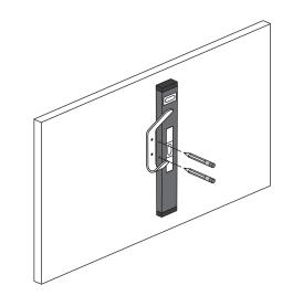
Drill a pilot hole for each marked location with a ¼" diameter drill bit. Install wall anchors into each hole. Be sure the lip of the anchor sits flush with the wall surface.
