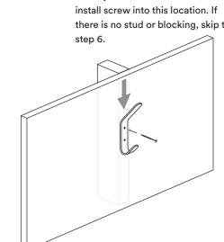
Level your most righteous hook, use a bullet level if needed. Mark the second hole with pencil or screw tip.
