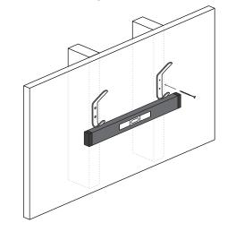
Install upper screw into marked location. Check for level, and install remaining screw into lower screw hole. Repeat for additional hooks. Skip to step 9.
