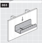
While the picture ledge is mounted to the wall, mark every remaining empty fastener hole with a pencil.
