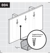
Remove the picture ledge from the wall to install wall anchors in each marked location that is not on a wall stud. Predrill each wall anchor location with 1/4" drill bit to avoid breaking wall anchors.
