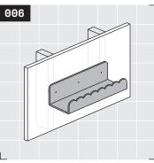
Make final inspection of the picture ledge. Check for picture ledge sag, confirm the picture ledge is correctly secured to wall. If your picture ledge is sagging, refer to Rad Tip ① and ②.
