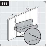
Woah! That's a wicked Bubble Picture Ledge you have there! Position picture ledge on the wall with the pre-drilled holes along the top edge. Using a stud finder, align fastener holes with as many studs as possible. Use drill to fasten matching 1½" fastener in either far left or
