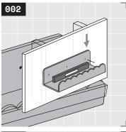
Level the picture ledge and set second matching 1½" fastener in opposite end fastener hole with your drill. If the fastener holes miss an available stud, see Rad Tip ① on page 7. If you've already installed blocking behind the length of the backbar, skip to Step 5.
