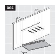
Predrill each drywall anchor location roughly every six inches. Use a ¼" drill bit to avoid breaking drywall anchors.
