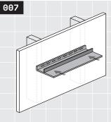
Install a drywall anchor in each of these pre-drilled locations. If you are using your own anchors, we recommend Toggler brand for best results. Stud locations should not be pre-drilled. Drywall anchors should be installed flush with the drywall surface.
