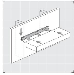
Begin sliding your shiny new hardwood shelf onto the bracket. Before pushing the wood shelf fully into place, insert wires into the 1/2" wall hole. See **Rad Tip ③**. At this point your electrician should already have a power supply and switch(s) installed, ready to
