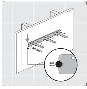
Replace bracket, drill fastener into each hole CO and confirm your bracket is correctly secured to the wall. See Rad Tip @ below. Each end of the steel bracket backbar has a half moon notch. Find the notch which aligns with the wired end of your shelf slab. Drill a hole through the wall inside this notch using a ½" drill bit.
