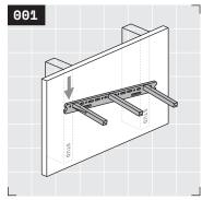
Let's dive in, homies! Orient your bracket on the wall so the channels across the top of your bracket face up. Use a drill to install a fastener in either far left or right hole. For more information on which fasteners to use, see **Rad Tip** ① on page 7.
