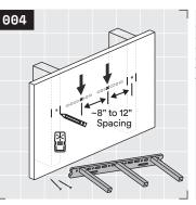
Use a stud finder to mark the location of every stud the bracket crosses. Then for areas between studs, mark one or two drywall anchor install locations roughly every eight to twelve inches or less along the length of the bracket depending on the stud spacing in your wall.
