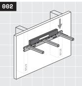
Level your bracket, set another fastener in the opposite end hole with your drill. If you have installed blocking behind the full length of your bracket, skip to **Step 6**. If you have not installed blocking, proceed to step **3**. For more information as blocking, and **3**. on blocking, see Rad Tip @ on page 7.
