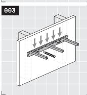
Mark all fastener holes and channels with a pencil. Once every fastener location has been marked, uninstall both fasteners and remove your bracket from the wall.
