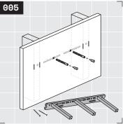
Predrill each drywall anchor location with a ¼" drill bit to avoid breaking drywall anchors. Install a drywall anchor in each of these pre-drilled locations. If you are using your own anchors, we recommend Toggler brand for best results. Stud locations should not be pre-drilled. Drywall anchors should be installed flush with the drywall surface with the drywall surface.
