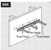
Confirm the position of the bracket and install a truss head fastener into every location crossing a stud or blocking. For every location that a drywall anchor was installed, ensure a fully threaded pan head fastener is used.
