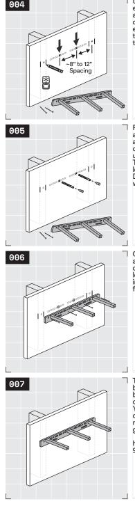
Use a stud finder to mark the location of every stud the bracket crosses. Then for areas between studs, mark one or two drywall anchor install locations roughly every eight to twelve inches or less along the length of the bracket depending on the stud spacing in your wall.
