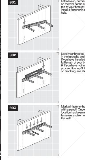
Let's dive in, homies! Orient your bracket on the wall so the channels across the top of your bracket face up. Use a drill to install a fastener in either far left or right hole.
