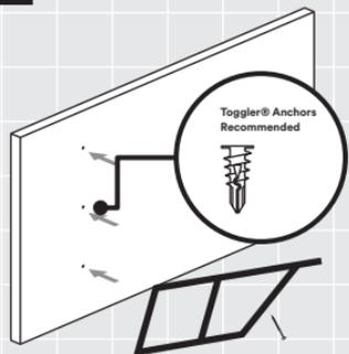
Remove the brackets from your wall. Predrill all marked fastener locations with a 1/8" drill bit, and install drywall anchors in each fastener hole location crossing drywall that isn't backed by studs or blocking. If you are installing on masonry, you must use a wall anchor rated for masonry use. If you are using your own anchors, we recommend Toggle brand. Take a swig of your brew.
