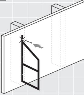
Yo, here we go! Position the first Verne bracket on your wall, ideally on a stud or blocking. See Rad Tip ① on page 7 if you don't know what blocking is. Mark the top-most fastener hole with the fastener tip. Remove bracket from wall, then grab a can of your favorite non-alcoholic brew and crack it open.
