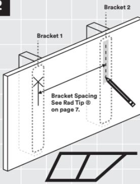
Measure the desired bracket spacing from fastener hole and righteously apply low-tack tape to general mounting area of second bracket. Measure again and draw a short vertical line on the tape. See Rad Tip ② on page 7.
