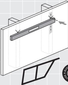
Place a level on first fastener hole. Find the intersection of the level and vertical line. If you do not have a long enough level, see Rad Tip ③ on page 7. Use a wall fastener to punch a hole into wall behind low-tack tape. Remove the tape.
