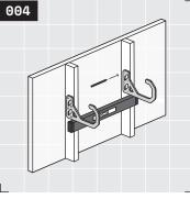
To mount additional hooks aligned with the first, use a level to align both hooks and repeat steps 1–3 with the second hook. See Rad Tip ②.
