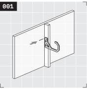
Yo! Here we go! Your Studly Hook is designed to be installed directly onto wall studs. See Rad Tip ① on page 7 for more information. Position your hook on a stud or post, then install a wall fastener into an upper fastener hole location.
