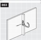
Install the remaining fasteners into remaining fastener holes. Your first Studly hook is installed! Crack open and take a swig of your favorite non-alcholic brew.
