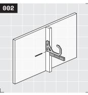
Straighten your hook using a level. Mark a lower fastener hole location with a fastener tip or a pencil. Install a second wall fastener into this location, then recheck for level.
