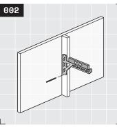
Straighten your bracket using a level. Mark a lower fastener hole location with a fastener tip or a pencil. Install a second wall fastener into this location, then recheck for level.
