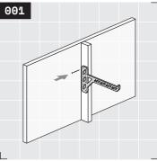
Yo! Here we go! Your Studly Bracket is designed to be installed directly onto wall studs. See **Rad Tip** ① on page 7 for more information. Position your bracket on a stud or post, then install a wall fastener into an upper fastener hole location.
