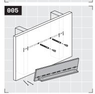
Predrill each drywall anchor location with a 1/2" drill bit to avoid breaking drywall anchors. Install a drywall anchor in each of these pre-drilled locations. If you are using your own anchors, we recommend Toggler brand for best results. Stud locations should not be pre-drilled. Drywall anchors should be installed flush with the drywall surface.
