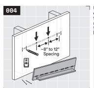
Use a stud finder to mark the location of every stud the bracket crosses. Then for areas between studs, mark a drywall anchor install location roughly every four to six inches along the length of the bracket.
