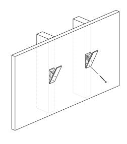
For installation into drywall only, 6 Position hook in desired location. Level the hook, and mark both screw hole locations with a screw tip.
