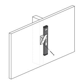
Install lower screw. You are done! When installing multiple hooks, see step 4 and 5, otherwise, skip to step 9.
