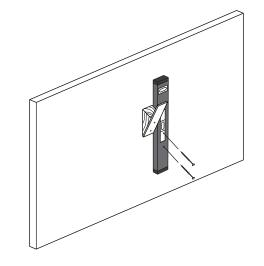
Drill a pilot hole for each marked location with a 1/4" diameter drill bit. Install wall anchors into each hole. Be sure the lip of the anchor sits flush with the wall surface.
