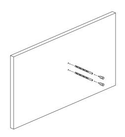
Install the hook making sure to use the longer screw for the upper location. See Rad Tip #3 below.
