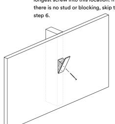
Level your most righteous hook, use a bullet level if needed. Mark the lower hole with a pencil or screw tip.
