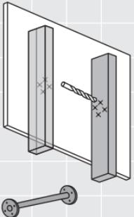
Use a  $\frac{1}{16}$ " drill bit to create a pilot hole at least  $1\frac{1}{2}$ " deep in the center of the mounting location before installing truss head fasteners.
