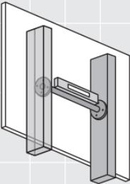
Once the structural support described in Step 1 has been established, hold the handle in desired location and use a bubble level to ensure straightness.
