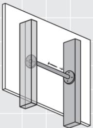
Install a truss head fastener through each mounting hole. Do not fully tighten until each fastener is in place. Once fasteners are installed, fully tighten each, checking for solid engagement between the fastener and the blocking or stud/joist.
