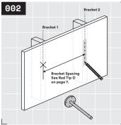
Measure the desired bracket spacing from fastener hole and righteously apply low-tack tape to general mounting area of second bracket. Measure again and draw a short vertical line on the tape. See Rad Tip @ on page 7.
