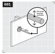
Yo, here we go! Position the first Roderick bracket on your wall, ideally on a stud or blocking. See Rad Tip ① on page 7 if you don't know what blocking is. Rotate bracket until set screw is oriented vertically. Mark the top-most fastener hole with a fastener tip. Remove your bracket from the wall, then grab a can of your favorite non-alcoholic brew and crack it open.
