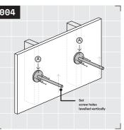
If top and bottom fastener holes are aligned on studs or blocking, install bugle head wall fasteners (②) in the top fastener hole locations. Vertically level each bracket to ensure shelf fastener holes in rods are pointing straight up. Punch a hole in all remaining fastener locations with fastener tip. See Rad Tip ③ on page 7 to ensure you are using the correct fastener.
