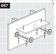
Slide the magnetic coverplates onto the rods to cover fastener holes. Lay the shelf slab on your brackets and position as desired. See **Rad Tip** ②. Hold the shelf steady and use a set fastener to poke a hole on the shelf. Remove shelf. Then, using a ½" drill bit, predrill set fastener locations ¾" deep (don't drill through the top of your shelf!) before installing the matching 1¾" set fasteners into the shelf.
