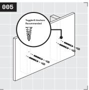
Fastener holes that are not on studs or blocking require a wall anchor. Remove the brackets from your wall. Predrill all marked fastener locations not crossing a stud or blocking with a ¼" drill bit, and install drywall anchors in each fastener hole location crossing drywall. Take a swig of your brew.
