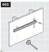
Place a level on first fastener hole. Find the intersection of the level and vertical line. Use a wall fastener to punch a hole into wall behind low-tack tape. Remove the tape.
