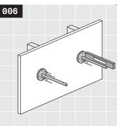
Position the brackets, install all wall fasteners. Review Rad Tip @ on page 7 to ensure you use the correct fastener to get the best function and most strength from of your bracket. Use a level to check each bracket for sag. See Rad Tip ® to remove sag. Confirm the brackets are secure to the wall.
