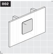
Partially install a fastener into an upper fastener hole location. Mark the location first with a pencil or fastener tip if needed. Do not fasten to full tightness.
