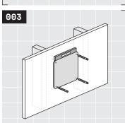
Level the board. Mark all remaining fastener hole locations. Uninstall the first fastener, and set the board aside.
