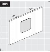
Yo, let's go! Position your Mosey magnet board on your wall, ideally with fastener holes aligned on a stud or blocking. See Rad Tip ① on page 7 for more on blocking.
