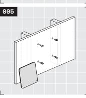
Install drywall anchors in each fastener hole location crossing drywall that isn't backed by studs or blocking. If you are installing on masonry, you must use a wall anchor rated for masonry use. If you are using your own anchors, we recommend Toggler brand.
