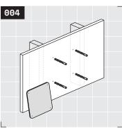
Drill a pilot hole for each fastener location using a ¼" drill bit. Pilot holes and wall anchors are not needed for locations backed by studs or blocking.
