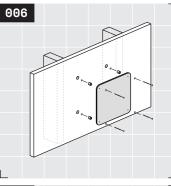
Position the board. Beginning at the top of the board, install all wall fasteners through board and nylon standoffs.
