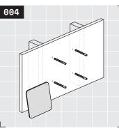
Drill a pilot hole for each fastener location using a ¼" drill bit. Pilot holes and wall anchors are not needed for locations backed by studs or blocking.
