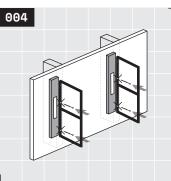
Install wall fasteners in the top fastener hole locations. Vertically level each bracket. Punch a hole in all remaining fastener locations with fastener tip. If your brackets are not on studs or blocking, skip to step 6. If your brackets are on studs or blocking, proceed to step 5.
