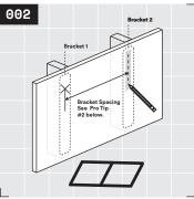
Measure the desired bracket spacing from fastener hole and righteously apply low-tack tape to general mounting area of second bracket. Measure again and draw a short vertical line on the tape. See Rad Tip ② on page 7.
