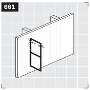
Yo, here we go! Position the first Lloyd bracket on your wall, ideally on a stud or blocking. See Rad Tip ① on page 7 if you don't know what blocking is. Mark the top-most fastener hole with the fastener tip. Remove bracket from wall, then grab a can of your favorite non-alcoholic brew and crack it open.
