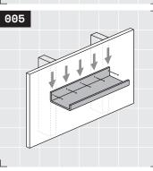
Replace the picture ledge. Drill matching 1½" fastener into each fastener hole.
