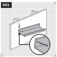
Woah! That's a wicked Fat Lippie you have there! Position picture ledge on the wall with the pre-drilled holes along the top edge. Using a stud finder, align fastener holes with as many studs as possible. Use drill to fasten matching 1½" fastener in either far left or right hole.
