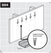
Remove the picture ledge from the wall to install wall anchors in each marked location that is not on a wall stud. Predrill each wall anchor location with ½" drill bit to avoid breaking wall anchors.
