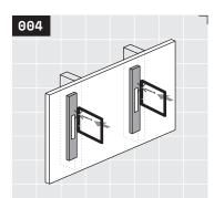
Install screws in the top fastener hole locations. Vertically level each bracket. Punch a hole in all remaining fastener locations with fastener tip. If your brackets are not on studs or blocking, skip to step 6. If not, proceed to step 5.
